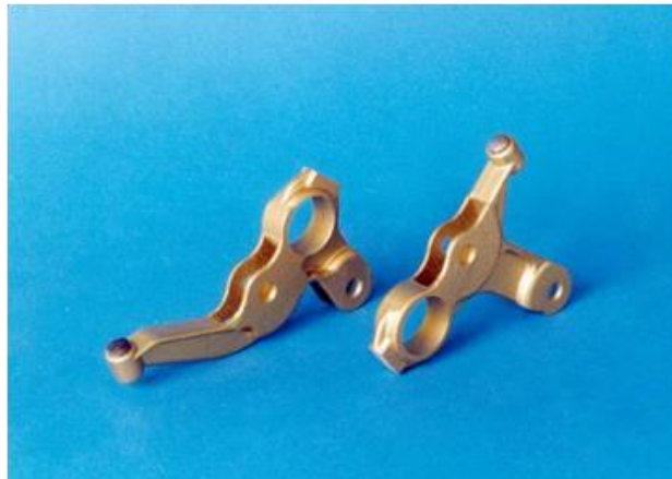
Fig. F5: Die cast roller levers with overmoulded steel bolt instead of a powder metallurgical MIM part
